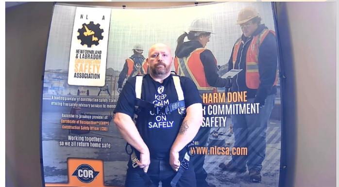
6. Check and adjust all straps. Once connected and buckled, adjust so that they are snug but allows full range of motion. Use loop keepers to keep hanging straps out of the way and check again that the D-ring is located between the shoulder blades.
